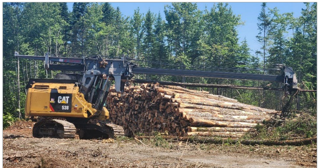
A stroke delimber processes and piles up tree-length wood for summer delivery in central Maine.
