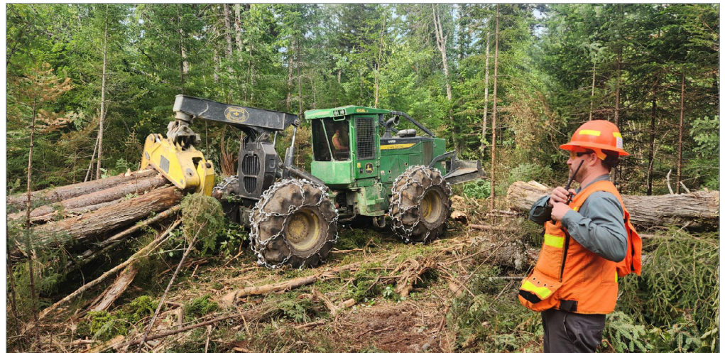
P&C forester Chris White monitors a grapple skidder carrying wood during a summer harvest in August 2025.
