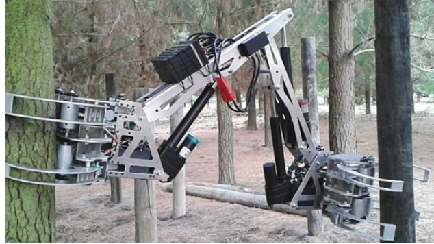
Figure 6. A Prototype Robotic Tree-to-Tree Felling Machine Under Development under New Zealand's Primary Growth Partnership. 18
